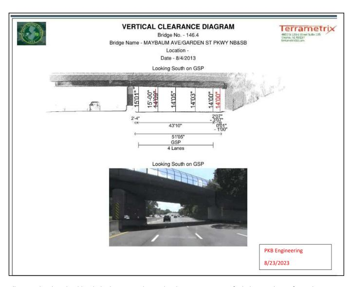
NOTE: All LIDAR sketches should include the Firm and Date the clearances were verified, this is to be performed during each NBIS inspection and during any Damage Inspections
