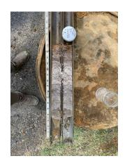
Accompanying the soil samples at each borehole location is a boring log describing the samples collected and providing other subsurface information required for design. The boring logs are reviewed by the engineer, and representative samples are selected and sent to a geotechnical laboratory for soil testing to confirm the field identification and determine engineering properties. Essential information collected from the geotechnical investigations will be utilized for the Final Design.
