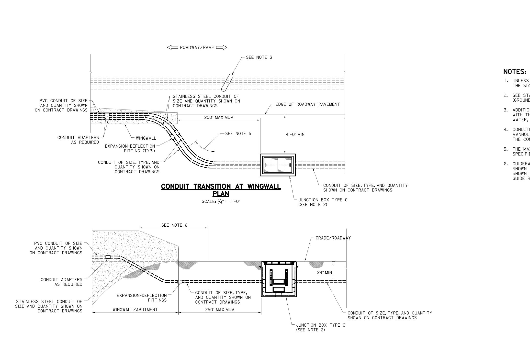
**CONDUIT TRANSITION AT WINGWALL ELEVATION** SCALE: <sup>3</sup>/<sub>4</sub>" = |'-0"
