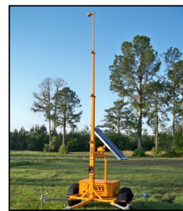
Figure 6. Camera and Solar Panel for "Smart Work Zone System."
