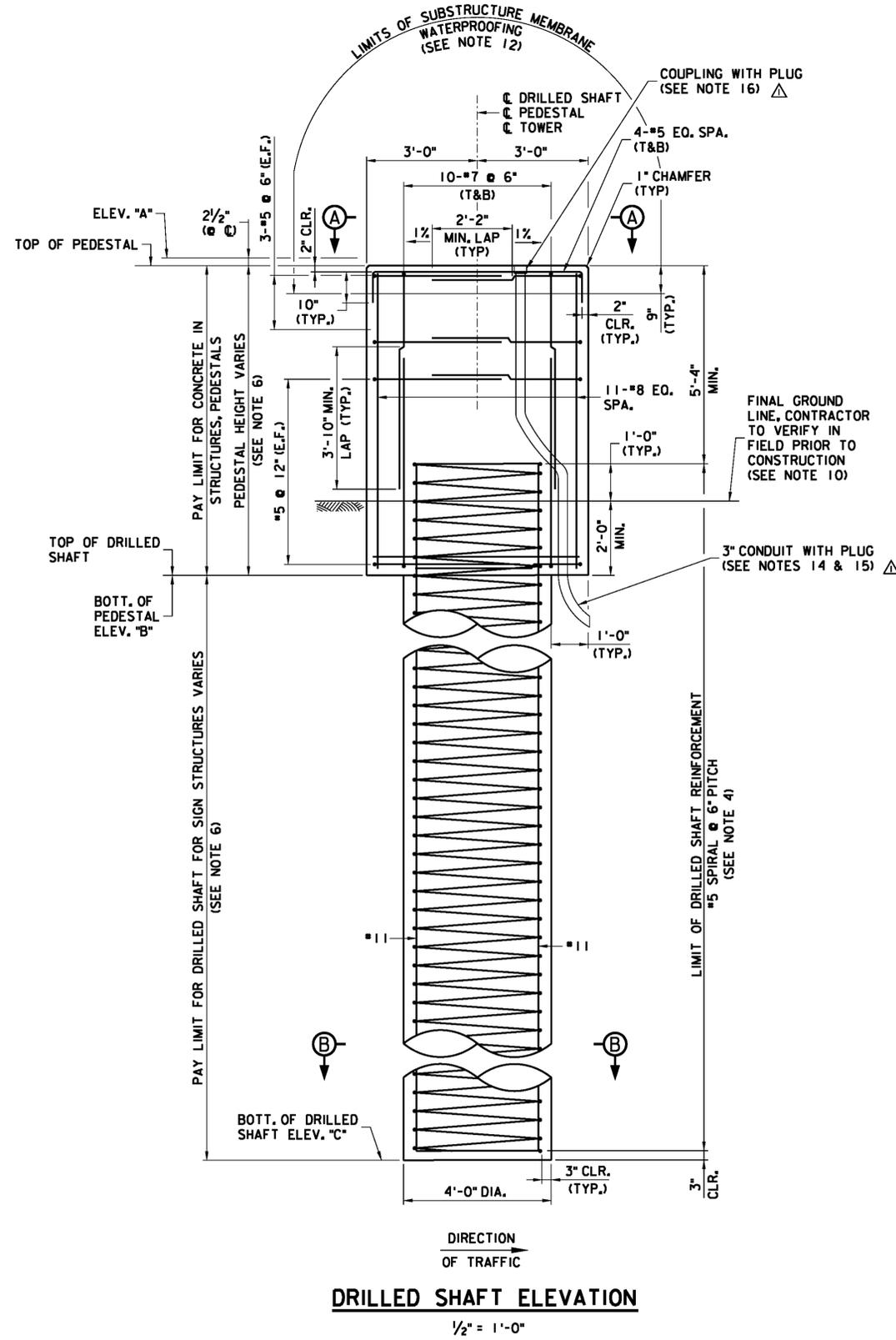
**DRILLED SHAFT ELEVATION**
