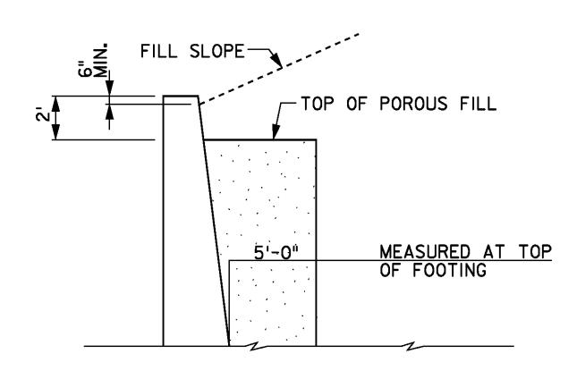
TOE OF SLOPE WALL SECTION
