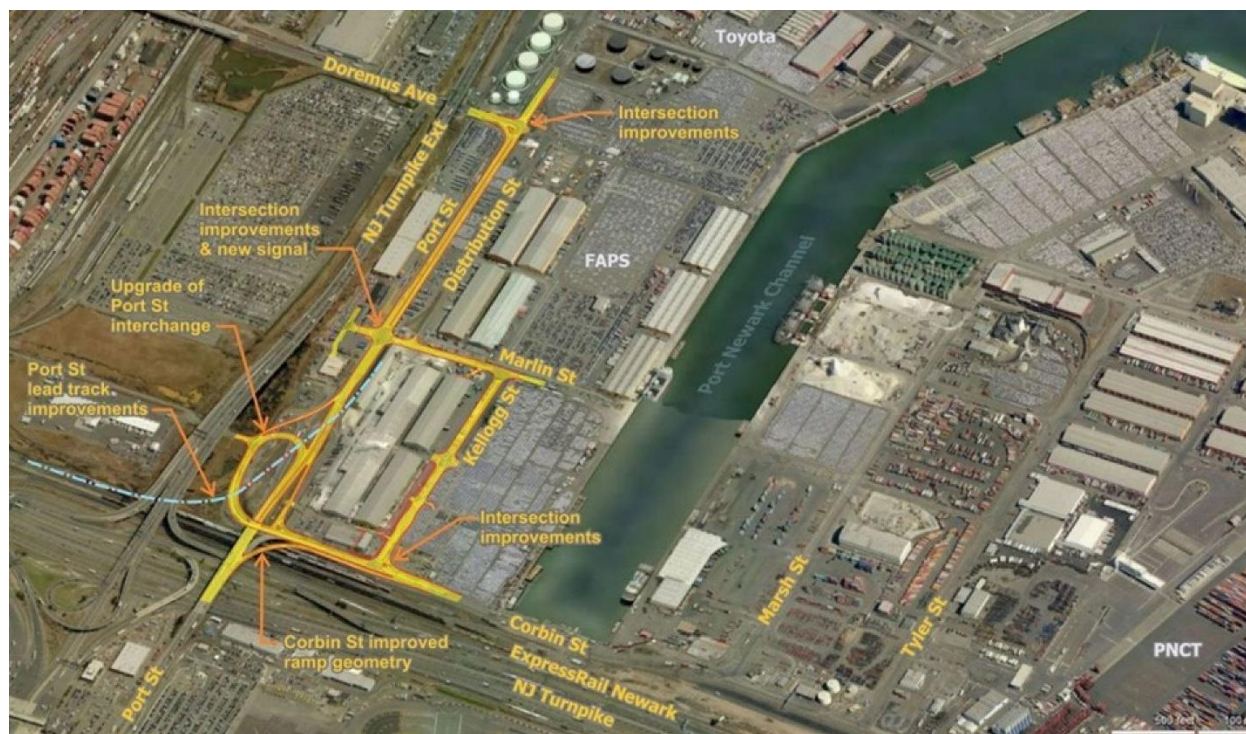
Figure 3.7-4. PANYNJ Port Street Corridor Improvement Project in Newark
